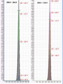
The CE for which maximum response was obtained was selected for each transition. Finally, 10 V and 20 V were selected for transitions 280.0 > 264.8 and 280.0 > 236.9, respectively. Transition 280.0 > 264.8 was selected as primary because it has highest m/z relationship and has more specificity.
