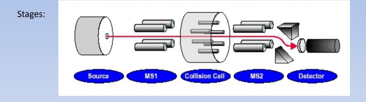
1) Analysis of the substances in Full Scan mode in order to obtain the MS1 spectrum and to select the precursor ion.
