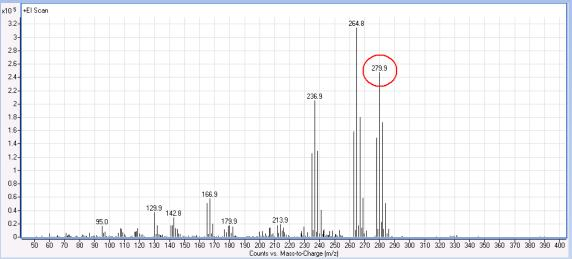
>90% correlation with the reference spectrum. Ion 279.9 was selected because it has a good intensity and the highest *m/z* relationship. The selected *m/z* corresponds to the molecular ion. Good response and highest selectivity will be obtained.
