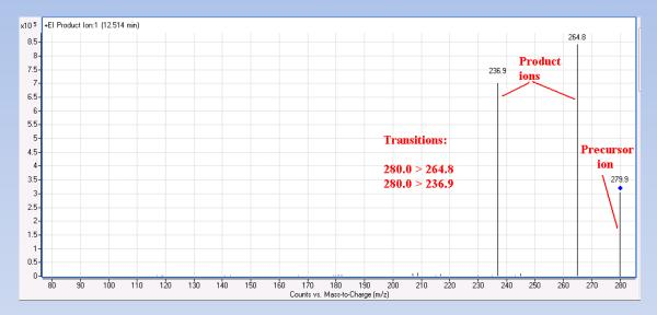
• Precursor ion 279.0 gave only two fragments, 264.8 and 236.9. They were selected as product ions and their optimal collision energy to obtain the maximum response was optimized.
